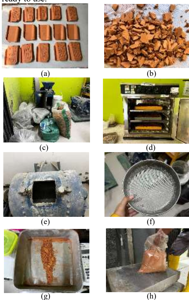
Figure 2. Preparation process of CRTWP: (a) natural drying; (b) manual crushing; (c) jaw crushing; (d) oven drying at 100°C; (e) grinding using a finish mill; (f)
