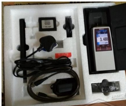
Figure-3. Mitutoyo SJ-2100 Surface Roughness Tester
