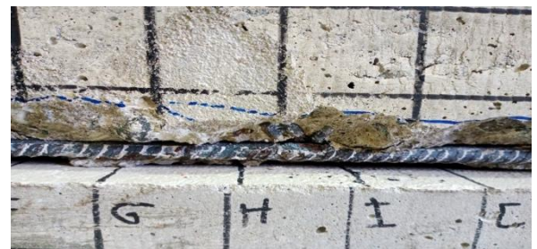
Figure-9. Cracks Observed in the STR G50 Reinforced Concrete Beam
