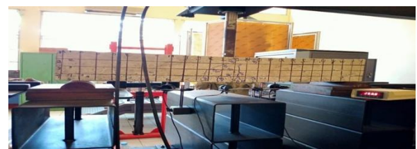
Figure-8. Cracks Observed in the STR G25 Reinforced Concrete Beam
