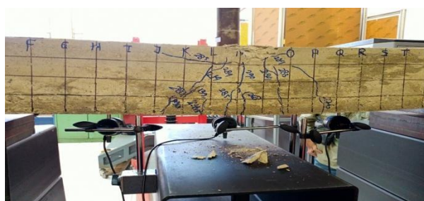
Figure-7. Cracks Observed in the STR T50 Reinforced Concrete Beam
