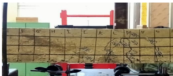
Figure-6. Cracks Observed in the STR T25 Reinforced Concrete Beam
