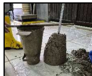
b). slump loss 2 (+30 minutes)
