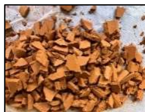
a). broken roof tile waste hammer
